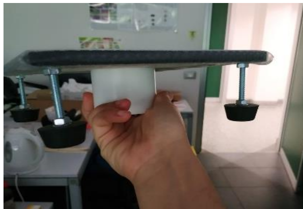
Picture 1: Vibro-plate is provided with 4 iron legs (h: 6.5 cm) and a mini-shaker is placed in the centre at the bottom of the plate (Photo: Valeria Fattoruso, Fondazione Edmund Mach)
