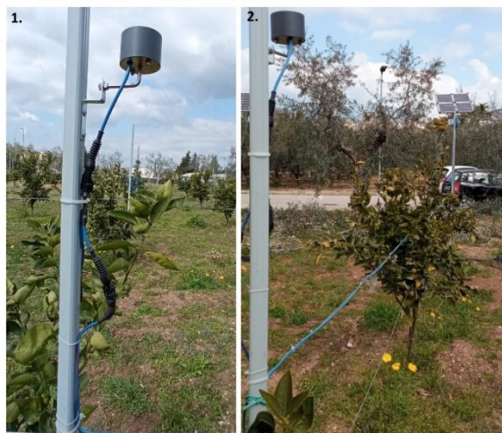
Picture 1: The mini-shaker is connected to the pole, and wires are in contact with the plants (Photo: Sabina Avosani, CIHEAM-Bari).
