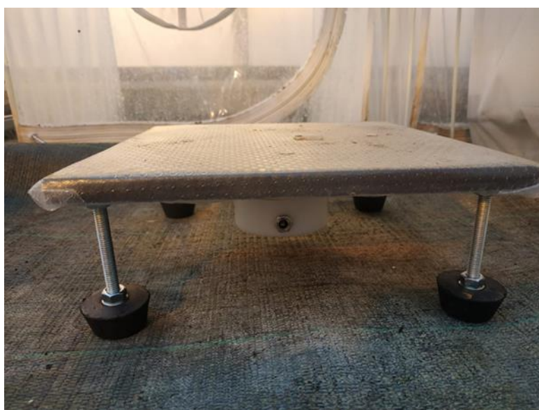
Figure 2: Vibroplate. Under the centre of the square plate on which the plants are positioned, a mini-shaker Tremos (CBC-Europe) which emits the disruptive vibrational signals.
