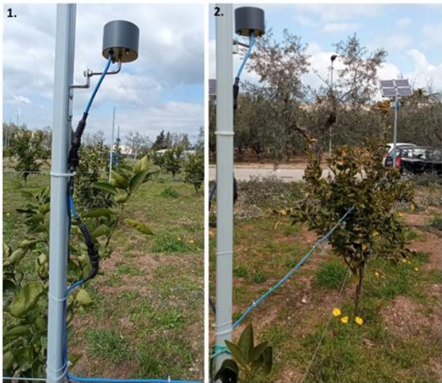
Figure 7: Left: the mini shaker is connected to the pole and the wires in contact with the plants. Right: citrus plants in direct contact with the wires that transmit the vibrations received from the pole and powered by solar panels (Photo of Sabina Avosani, CIHEAM, Bari)
